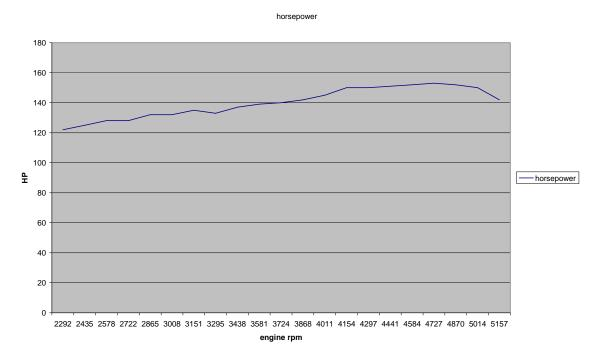
This graph is the HP output from that 308. It's measured at the wheels. No correction factor. Interesting Hp line huh!
