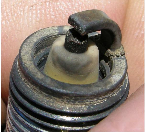
It is easy to see the damage to the center electrode and that the arc is blowing out to the outer shell of the plug. The intake valve is toward the back side of the photo. You need a powerful ignition to achieve this level of arc discharge and not get a misfire. This is a MSD 10 plus ignition. The engine did not misfire when arc blow out occurred but it changed exhaust sound and lost some power.
