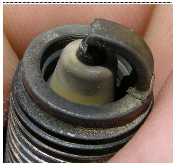
This plug is exhibiting arc blow. What is happening is the arc is being blown away from the electrode gap by extreme turbulence. You can see the arc blackness on the porcelain. The photos below is that plug from the other side. The index of the plug is such that the side showing in the photo below is facing the intake valve.
