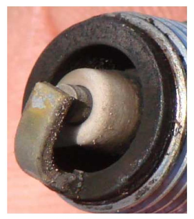
This is a plug from the same stuffed 308 but it's a high mileage general use photo. You can see the formation of tan graduating to dark grey at the base of the porcelain. This is unleaded street fuel. The mixture is leaner at the outer ring due to cruising AFR's etc.
